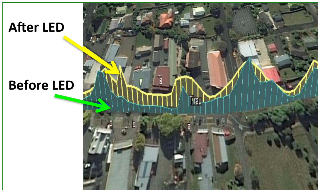
Figure 4 Mapping actual continuous street lighting performance instead of estimating it at single points (Source: Odyssey Energy)
