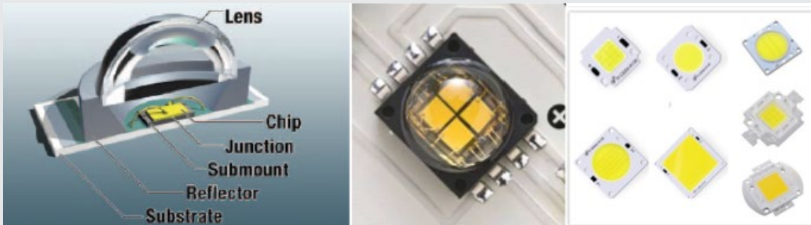
Figure 15 – Diagram and photos of Light Emitting Diode (LED) (CREE, US DoE)
